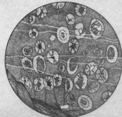
FIGURE 5. OIDS IN MUDDY MATRIX WITHOUT GROWTH APRONS White lines are fractures normal to section, spec. 203 B, deformation 30 per cent. Beekmantown (Ordovician) 2 1/4 miles SE. Greencastle, Pa., road to Leitersburg, Md.
